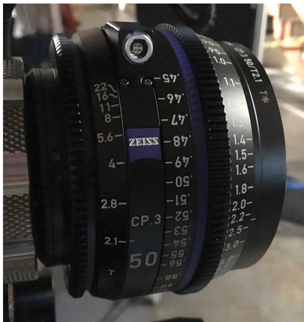
FIGURE 4. A shot of a new Zeiss CP.3 xD 50mm T2.1, the follow up to the incredibly popular Zeiss CP.2 line. The xD version of the CP.3 is the "Extended Data" incorporating the Cooke /i metadata system and incorporating open data cells to include lens-specific distortion and vignetting data that can be dialed out in post with the literal toggle of a menu option. The evolution of smart lens metadata leads us to a day when visual effects artists no longer have to shoot distortion and shading tests for every lens used on a job. Zeiss has made that obsolete with the CP.3 internal data.
